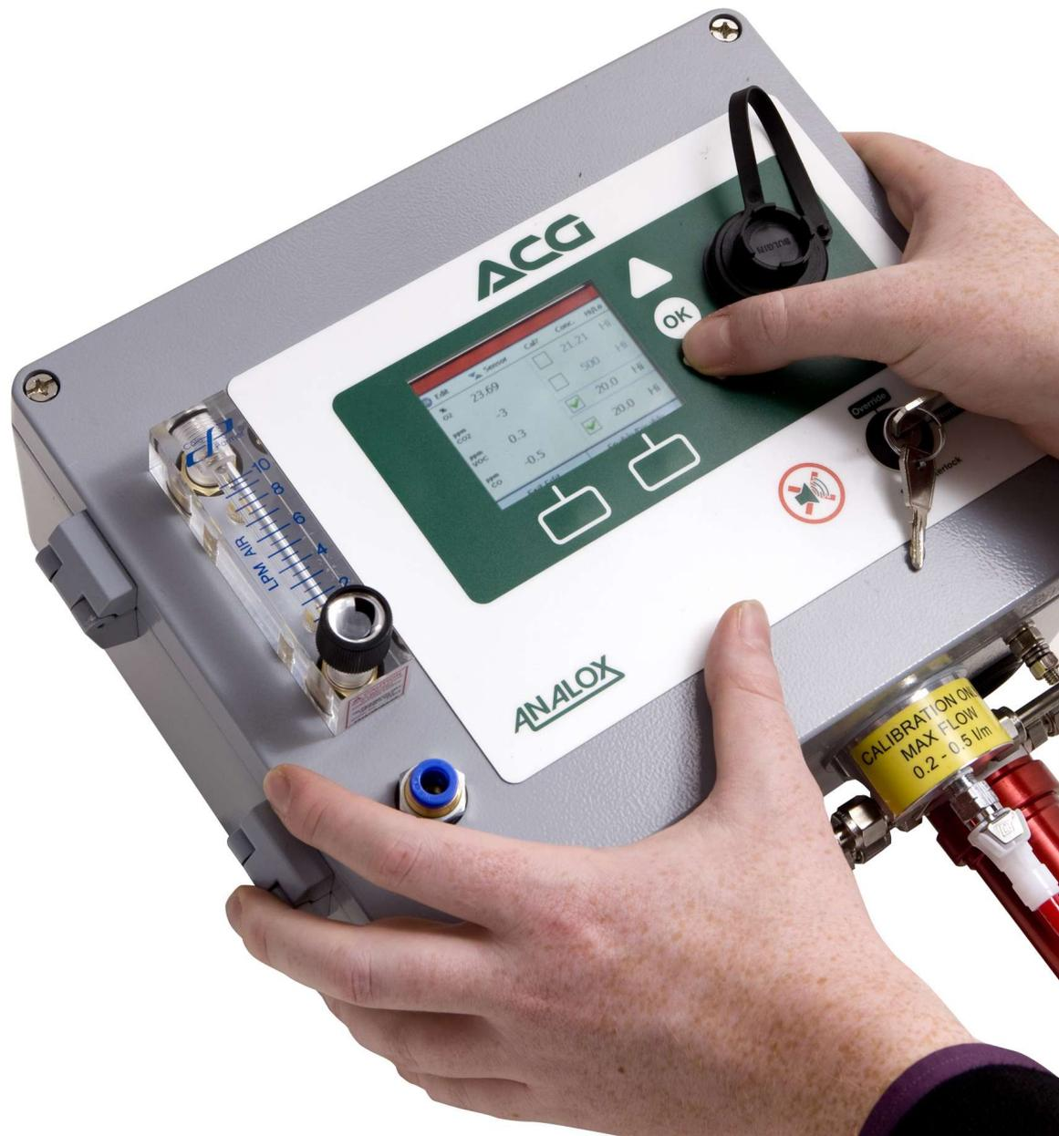
Real time continuous monitoring of contaminants in compressed breathing air
