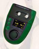
The Aspida is a personal, portable alarm ideal for protecting your staff from O<sub>2</sub> depletion dangers in fumigation or cargo areas. It is available in three different versions, O2 only, CO2 only or a dual monitor which monitors O2 and CO2. The unit is equipped with many different features including a mandown alarm which is perfect for lone workers, data logging and battery flexibility. If you don't have time to charge the Aspida, simply add 2 x AA batteries for instant power.
