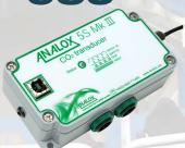
The 5S3 is a dual beam IR (Infra Red) CO2 sensor which is ideal for monitoring CO2 levels inside the silo bins to help prevent spoilage. The 5S3 is supplied in an aluminium enclosure, has a 5 wire connection and can offer 4-20mA or 0-2V output. This sensor can be linked to our MCU control panel to provide displays, alarms and datalogging.
