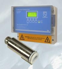
The LC Commercial control panel and 3000si O2 sensor combination provides complete multi point monitoring, ideal for larger sites. The LC Commercial allows users to view the readings and status of all the sensors from a single point. It also provides a 4-20mA signal for integration into BMS (Building Management Systems) and relay outputs for each sensor channel which can be used to trigger extraction systems, beacons or system shutdown.
