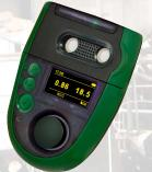
The "Livestock Aspida" can be cited at animal level and give continual readings of CO<sub>2</sub> & NH<sub>3</sub> and audio visual alarms should permissible levels be exceeded. The unit also datalogs and information easily retrieved through a USB connection. It can be used as a portable or fixed
