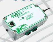
The 5S3 is a dual beam IR (Infra Red) CO2 sensor which is ideal for monitoring CO2 levels inside the glass house to ensure the best possible conditions for the yield. The 5S3 is supplied in an aluminium enclosure, has a 5 wire connection and can offer 4-20mA or 0-2V output. This sensor can be linked to our LC Commercial control panel to provide displays, alarms and outputs.
