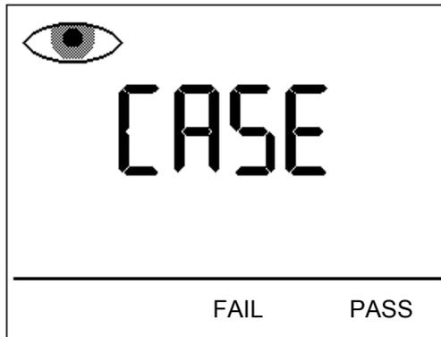
Recording a fail result will cause the tester to skip testing and go straight to the end of test options.
