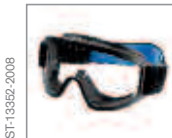
Safety goggles Black, visor of polycarbonate (2 mm), anti-scratch and anti-fog coating, optical class 2 and ballistic protection class B, accor. to EN 166 R 56 076
