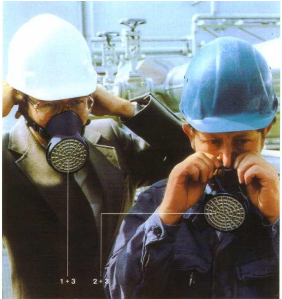
In case hazardous substances are present at a work place it has to be taken into account that all of a sudden they occur in concentrations that cause severe health impairment or even death. Then the filter escape units Parat 1 and Parat 2 have a single but vital task to perform: They have to ensure that user is provided with protection along his escape route into a safe, breathable atmosphere. Therefore they are tailored to compactness, robust design and safe handling.
