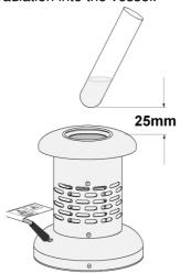
7.2.5. For quick heating, the test tube should be positioned so that it is just inside the mouth of the ceramic heating bowl.
