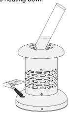
7.2.6. Non-contact crucible heating may be achieved by removing the cowl. It is recommended that heat resistant gloves should be worn when removing the cowl). The cowl is removed by rotating in the direction indicated in the illustration below.
