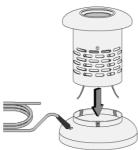
9.2.3.Unscrew the terminal block positions and remove the fuses. Fit replacement fuses of the correct rate and value.
