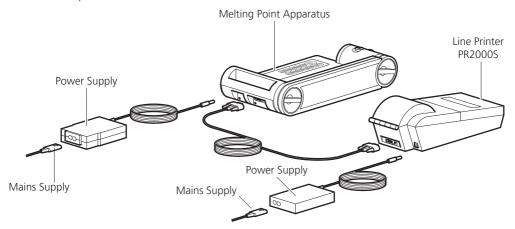
The PR2000S serial printer is set up for compatibility with the IA. The Baud rate on the PR2000S printer is factory set at 9600.
