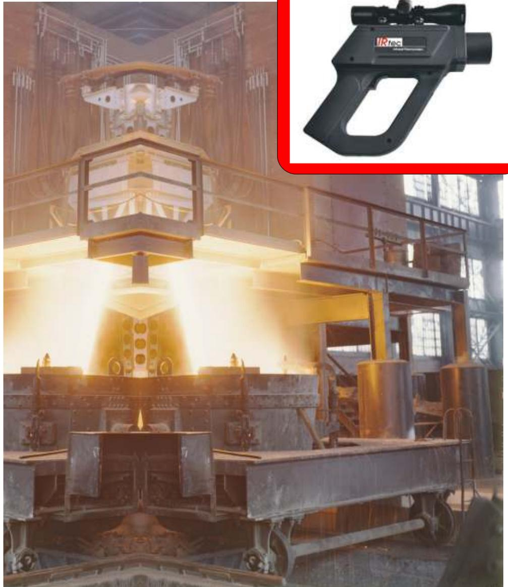
Each body, at temperatures above the absolute zero (-273°C or 0K), emits energy as electromagnetic radiation. When temperature rises, the intensity of this infrared energy increases. The temperature of the body surface can therefore be determined by measuring the intensity of this energy in a small spectral band: the infrared region. The instruments used to measure this energy and to calculate the related temperature are called infrared thermometers or non-contact thermometers.
