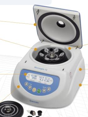
Microspin 12 with fixed angle rotor for 12 x 1.5/2 ml microtubes
