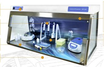
Built-in UV cleaner - recirculator both increases the maximum density of UV light and generates 25 m3/h air flow exchange prevents unwanted contamination and protects the user from direct UV light (in the upper hood) during manipulation
