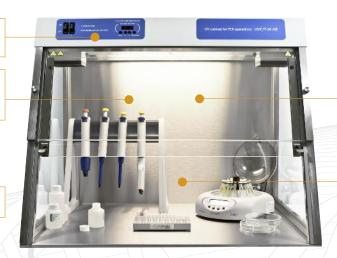
Built-in UV bactericidal cleanerrecirculator (patented) both increases the maximum density of UV light (in the upper hood) and generates 25 m<sup>3</sup>/h air flow exchange - prevents unwanted contamination and protects the user from direct UV light during manipulation
