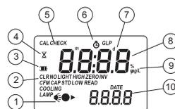
1. The measuring scheme (lamp, cuvette, detector), appears during different phases of zero or reading measurement
