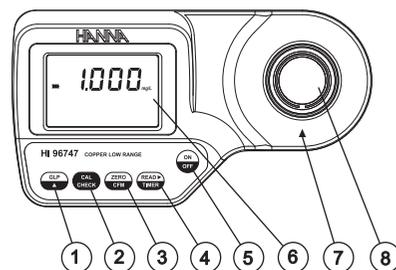
1. **GLP/** key: press to enter *GLP mode*. In *calibration mode* press to edit the date and time.
