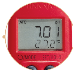
Simultaneous display of pH and temperature
