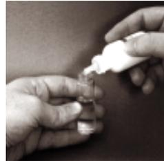
**Note:** In order to minimize any error introduced by the cuvette, it is recommended to use, during calibration, the same cuvette you are going to use to perform the measurement.
