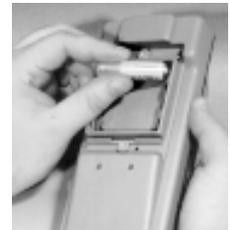
After the batteries have been installed, close the battery cover and tighten the 2 screws.
