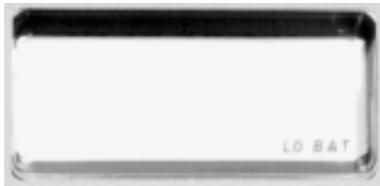
A "**-BA-**" indication will appear on the display when the batteries are too weak to perform reliable measurements. The message appears for a few seconds, and then the meter will automatically switch off. Batteries must be immediately replaced.
