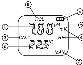
1. Main display - 3½ digit display providing direct readout of pH or mV. Underrange (-1) and Overage (1) symbols will be displayed if the instrument is reading outside the ranges of:
