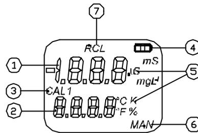
1. Main display - 3½ digit backlit LCD providing direct readout of conductivity (in  $\mu\text{S}$  or  $\text{mS}$ ) and total dissolved solids (TDS) (in  $\text{mg/l}$  or  $\text{g/l}$ ). The display will also show Underrange (-1) and Overage (1) symbols if the instrument is reading outside the operating ranges.
