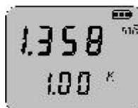
The ▲ ▼ keys can then be used to adjust the cell constant to the value indicated on the conductivity cell being used.
