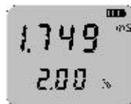
Adjustment of the coefficient may be made by selecting % on the secondary display using the MODE key and then using the ▲ ▼ keys to set the required value.
