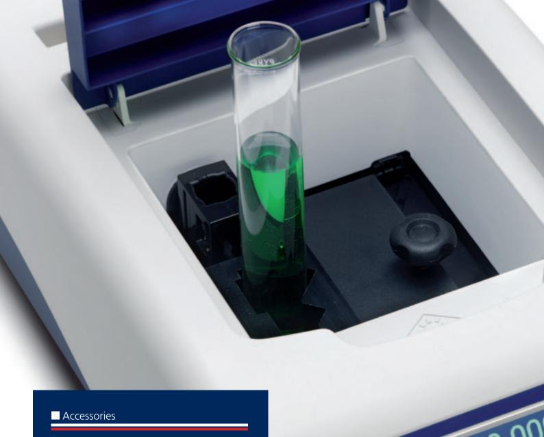
The 72 series spectrophotometers have been designed to be compatible with the extensive range of accessories already available from Jenway. These include a test tube holder, adjustable path length (10 to 100mm) cuvette holder and a microcuvette holder. All of the accessories are easy to interchange using the ergonomic thumb screw.
