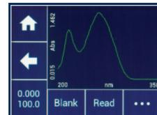
Where nucleic acid concentrations are high, or there are only small sample volumes available for testing, there is a dilution option which can be used to calculate the original concentration of diluted samples.
