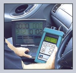
The Kane Auto 4-1 & 5-1 Series Exhaust Gas Analysers are truly portable and set new standards of convenience and ease of use. Weighing just 1kg, the handset fits comfortably in the hand and can run for up to 4 hours on its internal re-chargeable battery.
