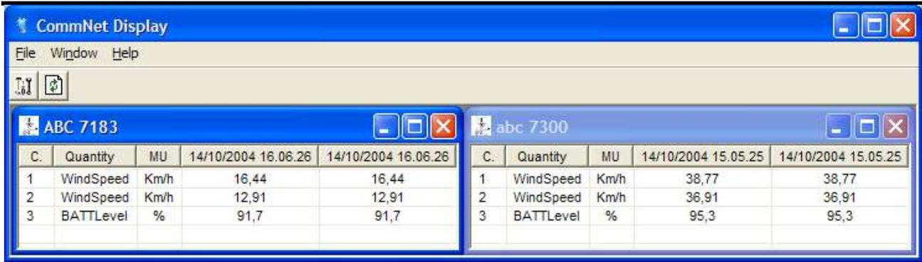
If *CommNet Display* has the updating rate lower than the calling rate programmed in CommNet, the two columns with the instantaneous values could be identical.
