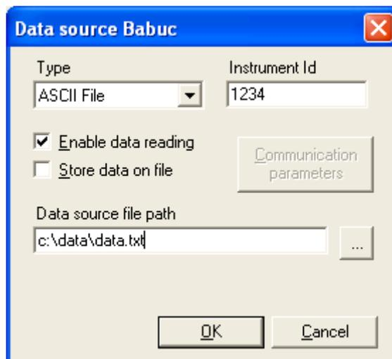
Setting example for the data reading from one instrument configured in CommNet.
