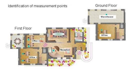
In a situation of this kind, the thermal project will include two main areas, the *ground floor* and the *first floor*; each of these areas (named *Site* in the program) it contains few other spaces (*Office* and *Warehouse* on the *Ground Floor*, *Office 1*, *Office 2* and *Reception* on the *First Floor*); each of these areas will cover one or more measure points where the calculations will be carried out.
