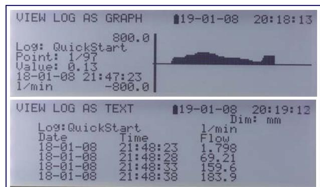
If logging is taking place at a 'named site' the log is saved with same 'name' as the site name and can be recalled under that name as and when required. This allows the instrument to be used at several site locations and the results can be downloaded independently at a later, convenient time.
