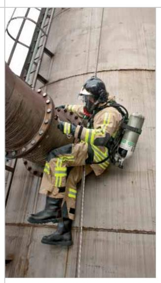
Applications that require both SCBA and fall protection are always challenging for the user. Putting a breathing apparatus on top of a fall protection harness is time-consuming when it comes to donning and uncomfortable in use.
