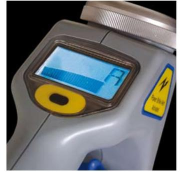
In AvoidanceScan™ Mode P, R and G operate simultaneously providing faster surveys.
