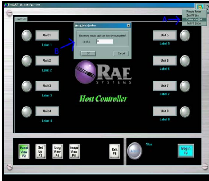
Figure 3. Advanced Tools>>Define Max Unit. Select the 'Define Max Unit' from the 'Advanced Tools' bar (A), and proceed to select the number of units the controller will attempt to communicate with (B).
